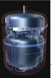
The cryostat vacuum vessel containing the superfluid helium tank. The gas is ejected into space. The cryostat vacuum vessel is cooled down to about 70K ( $-203^{\circ}$ C) by radiating heat into space.
