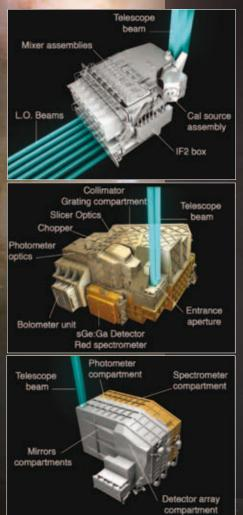
The Heterodyne Instrument for the Far Infrared (HIFI), a high-resolution spectrometer, is designed to observe unexploited wavelengths. With its high spectral resolution – the highest ever in the
