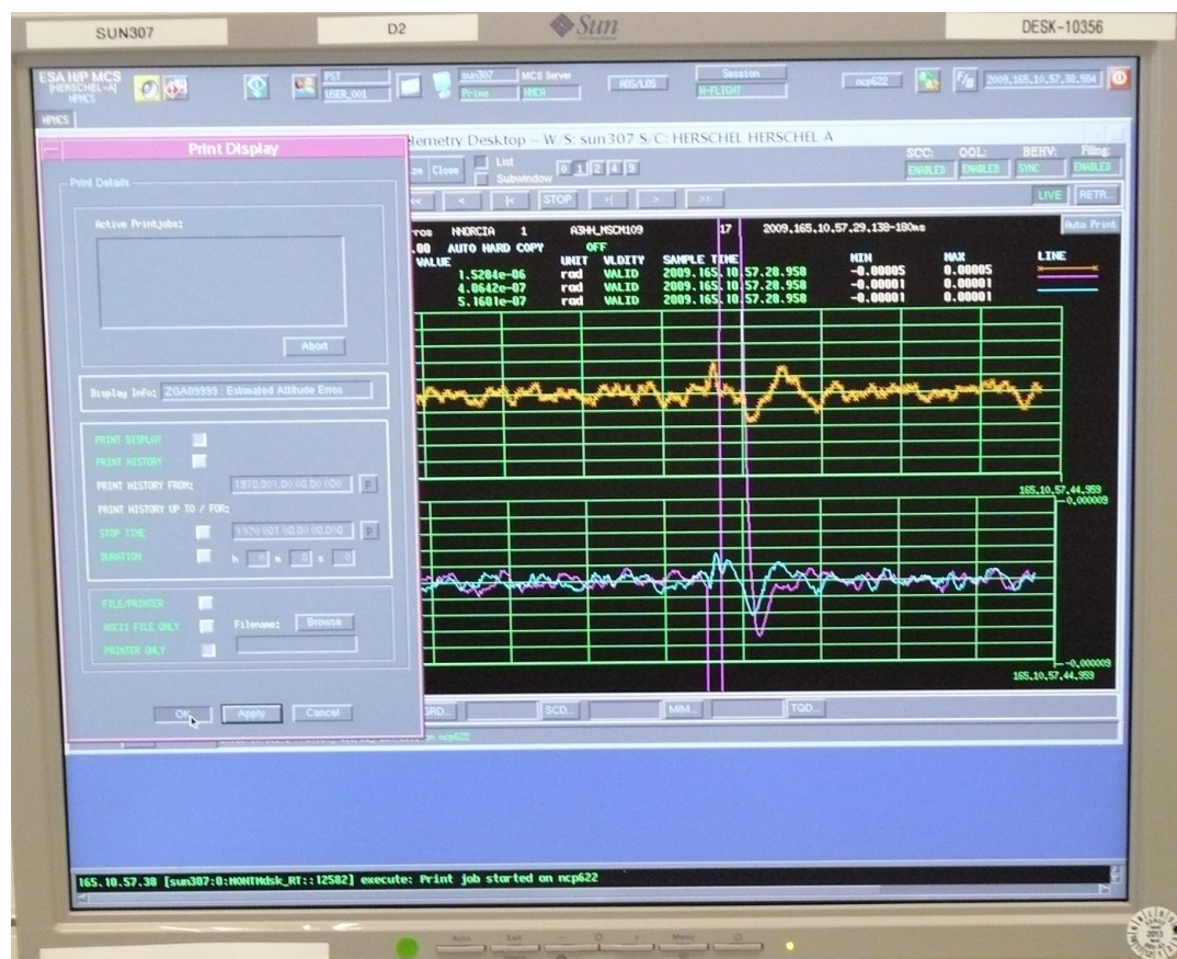
Figure 1.4. The telemetry received at MOC showing the oscillation in gyro response as the heavy cryo-cover swung open and oscillated, causing the entire satellite to wobble slightly until it had reached a stable open position. This gyro signal was the first evidence that the cryocover opening had been carried out successfully.
